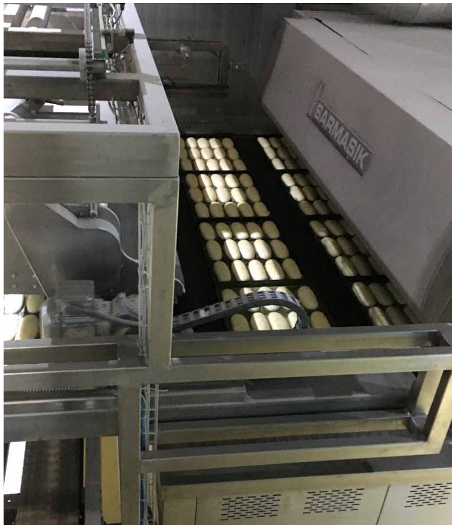
Trays pass through a sprayer and then into a Sarmasik tunnel oven.
